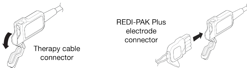
Figure 36 Connect QUIK-COMBO Electrodes to Therapy Cable
